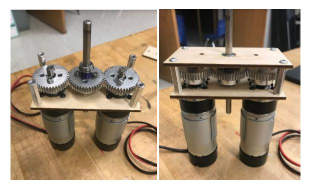
This is the final gearbox. At first, the gears were extremely tight and didn't run smoothly. To solve this we loosened the motor screws and used the extra tolerance to pull the motors apart slightly before tightening the screws again.
