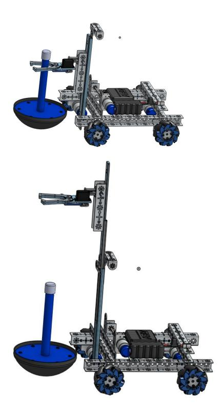
Another arm design idea that was thought of was a sideways elevator. This is similar to the current elevator, but it has different packaging than the current design. The idea could be considered if the center space is needed for other systems. A quick sketch of the arm on a lift shows the possible configurations.
