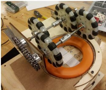
For the collector we were able to assemble it and attach it to the robot. After some testing, the only concern is one that was already brought up. The design only works when the bottom roller is spinning. This just means that we will need to power it with something better than a rubber band on the final version.
