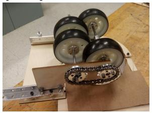
But the omni wheels seem to work okay, as they are thinner. While there are some benefits of the omni wheels (loading the discs is slightly easier), the wheels seem to slip a little. This is detrimental to our design because it relies on the wheels ejecting the disc as fast as possible. Our plan for this is to keep testing this to substantiate this concern.
